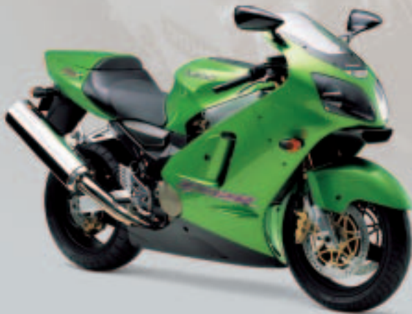
2000 ZX1200-A Ninja ZX-12R 4-stroke Liquid-cooled In-Line Four DOHC, 16 valves 1,199 cm 3
